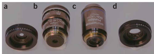
Figure 3 | Accounting for differences in the objective back aperture. (a) Calibrated iris with 5-mm opening. (b,c) Photograph of two different high numerical aperture objectives. The open apertures of the objectives are largely different. (d) Calibrated iris with 12-mm opening. If the iris is placed at approximately the same relative position within the beam (Fig. 2b) as the aperture of the objective, it can be used to selectively measure only the amount of light that is actually entering the respective objective.
